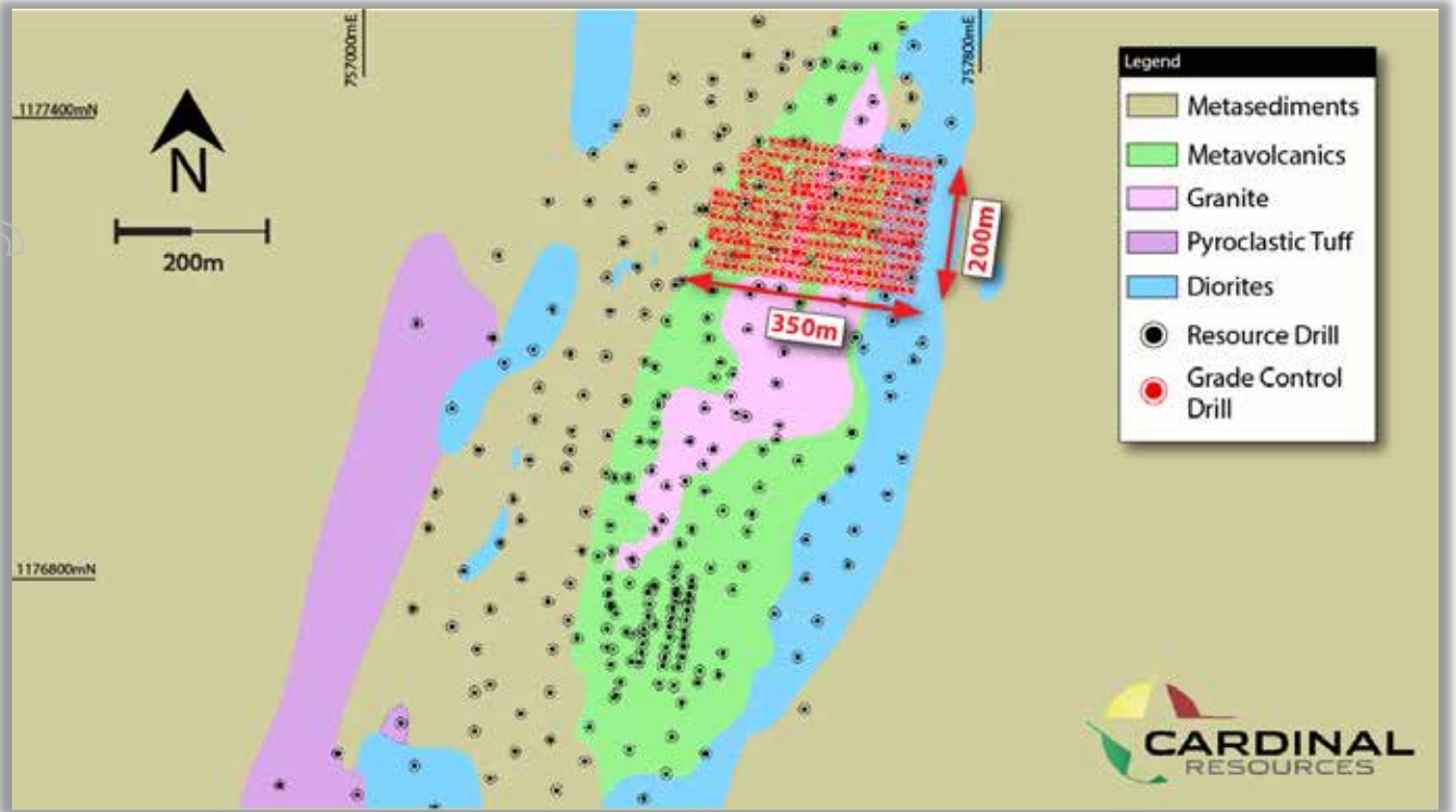
Figure 2: Plan View of Namdini deposit showing drill hole locations and interpreted geology
