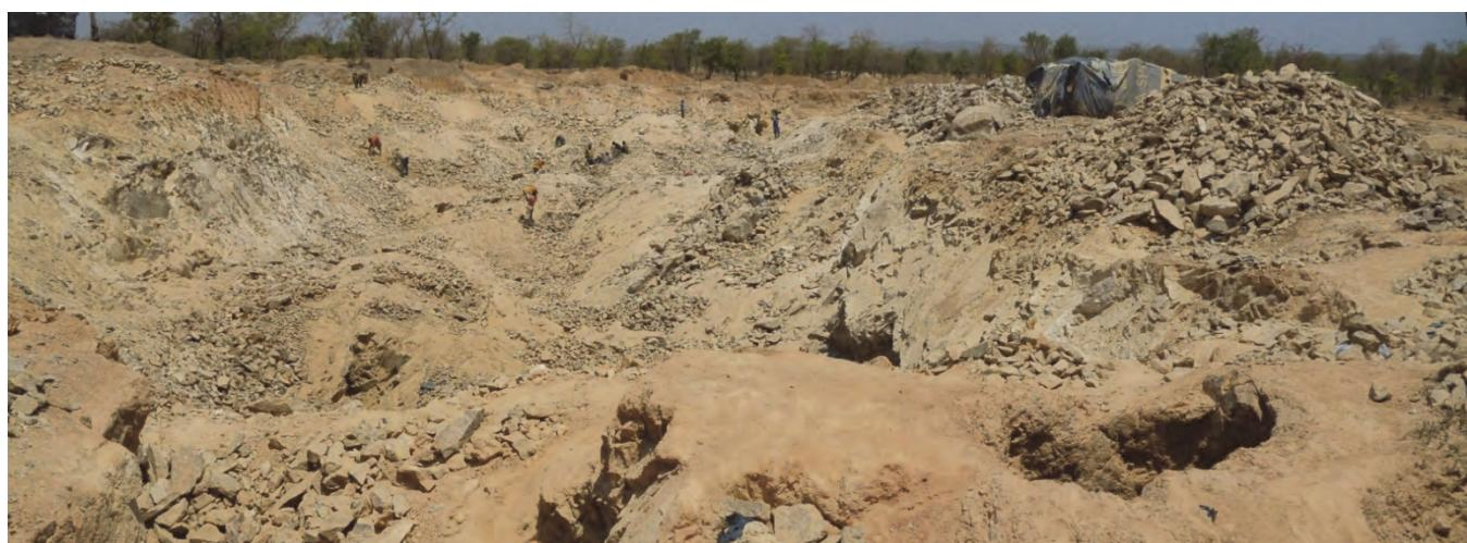
Figure 3: Active artisanal workings in monzonite granitoid
